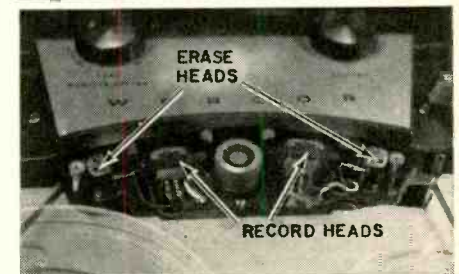
Fig. 8—Two closeups of recording and erase heads.
