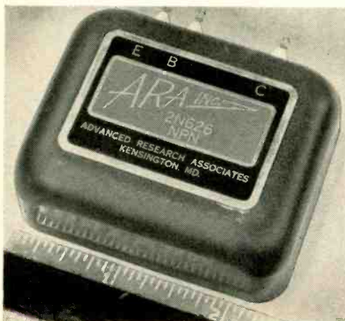
Type 2N626, a germanium n-p-n composite transistor.
